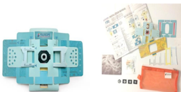
Figure 1. Foldscope - the Origami Paper Microscope.
